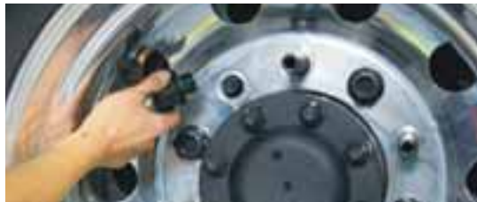
STEP 7 Install the nuts by hand.
